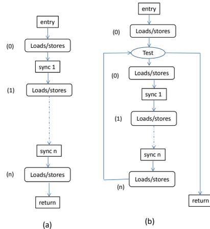
**Figure 3: Structure of thread start functions suitable for phased thread section analysis. (a) Straight Line (b) Looped**
