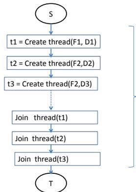
Figure 1: A typical threaded section of program
