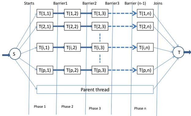
**Figure 2: A decomposition of threaded section into smaller, disjoint parallel phases**
