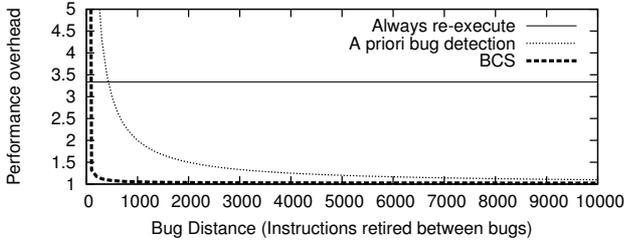
Figure 6: Slowdown for different techniques to tolerate bugs
