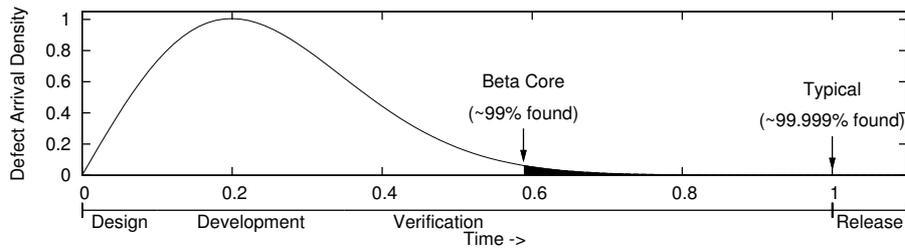
**Figure 1:** Defect arrival model using a SLIM model [10].
