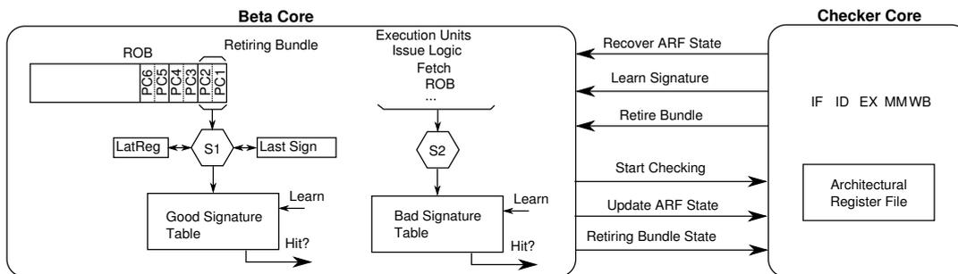
**Figure 3:** Beta Core Solution integrating an out-of-order Beta Core and a simple in-order Checker Core. LatReg is the latency register indicating the number of cycles since the last retirement. S1 and S2 are the signature generators for the good and bad signatures respectively.
