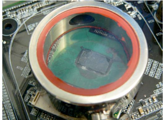
**Figure 9: Transparent sapphire heat sink.**
