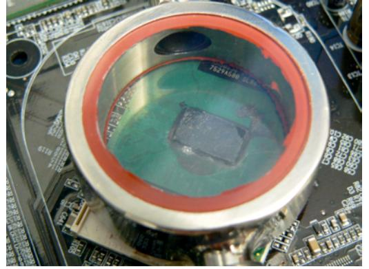
**Figure 9: Transparent sapphire heat sink.**
