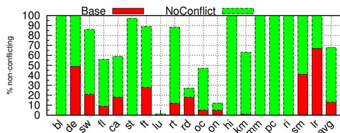
Fig. 6: Reduction in dynamic load instrumentation by SBPA. 68% of loads were identified as non-conflicting on average, with few applications reaching 100%.
