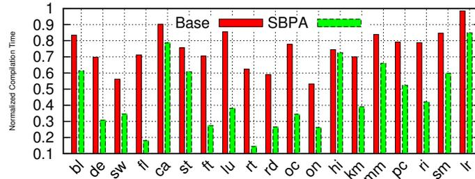
Fig. 10: Compilation times of Base and SBPA normalized to compile times when no optimization is applied. On average, Base was 75% and SBPA was 46% of unoptimized compile times.
