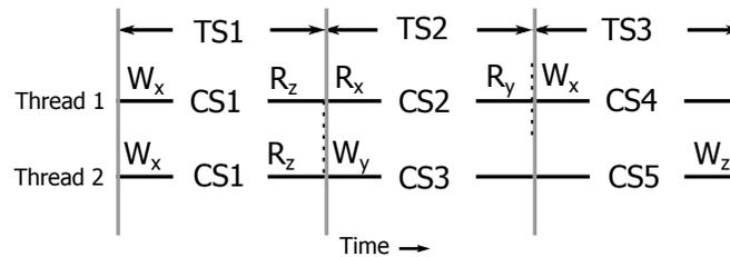
Fig. 3: Two threads executing 5 code sections in 3 disjoint thread sections.
