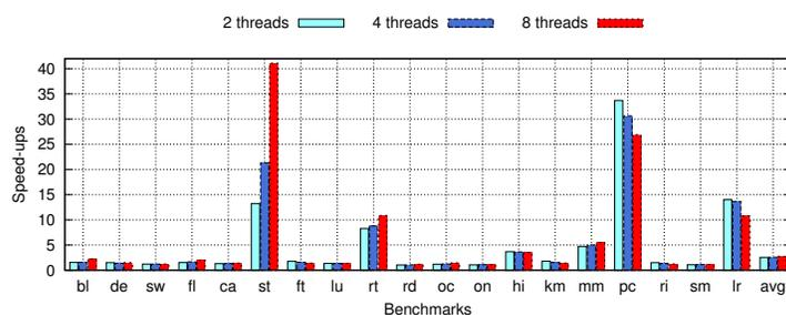
Fig. 8: Geometric mean speed-ups of ThreadSanitizer instrumented executables with various options.
